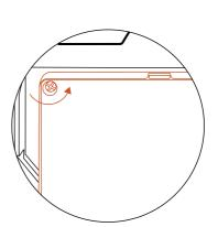
**3.** Loosen the 4 screws holding the battery. compartment in place with a cross-tip screwdriver.
