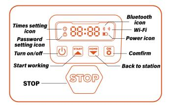
Power icon: The battery power icon shows the remain power of the machine. This icon displaying 1 bar indicates that the power is 30% or under, displaying 2 bars indicates that the remain power is between 31-66%, and displaying 3 bars indicates power of 67% and higher.
