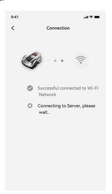
**Step 2:** Configure your Wi-Fi for the machine in the app. The machine needs to be connected to the same Wi-Fi as your mobile phone. Enter your home WiFi name and password. ( If your mobile phone has connected to Wi-Fi before scanning the QR code, the app will automatically capture the Wi-Fi name, otherwise you need to enter the Wi-Fi name manually.)
