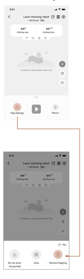
> Select the corresponding robot in the app to enter the machine control panel and click "Map Settings" icon to enter the map building panel. Choose the "Remote Mapping" function to start controlling the mower remotely and creating the map.
